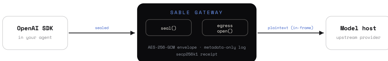
FIG. 1 – THE SEALED PIPELINE. PLAINTEXT EXISTS ONLY BETWEEN OPEN() AND THE UPSTREAM CALL.
